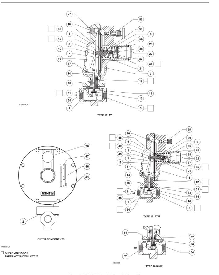
Figure 7. 161AY Series Monitor Pilot Assembly
