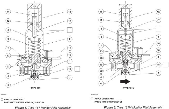
Figure 4. Type 161 Monitor Pilot Assembly
