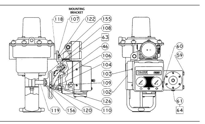
Pneumatic tubing connected to the DVC5000 brings instrument supply air to the DVC5000 and takes controlled output air from the DVC5000 to the actuator. The pressure sensor in the DVC5000 measures the output pressure and presents it as a device variable.
