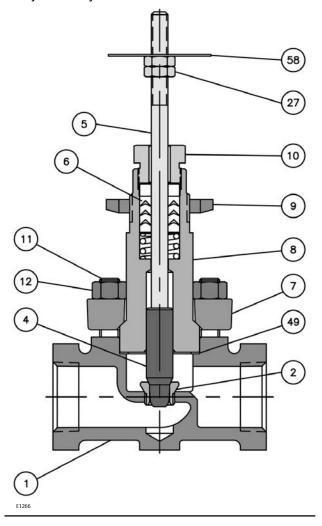
Figure 3. Baumann Flangeless (NPT) Threaded Valve Body Assembly with Single Extension Bonnet
