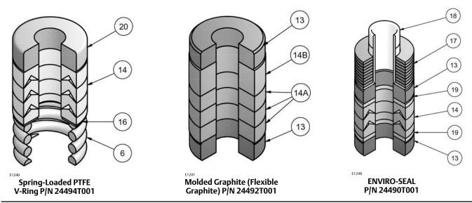
Table 9. Spring-Loaded PTFE V-Ring Packing Kit P/N 24494T001
