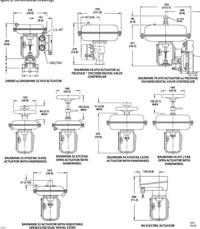
NOTE: ACTUATOR REMOVAL REQUIRES 115 mm (4.5 INCHES) VERTICAL CLEARANCE.
