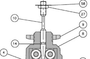
Figure 7. Baumann 81000 NPS 1/2 Inline Valve Body
