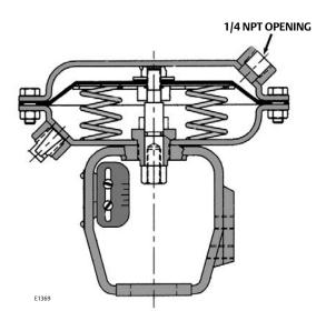
Figure 3. Air-to-Retract (Air-to-Open Action)
