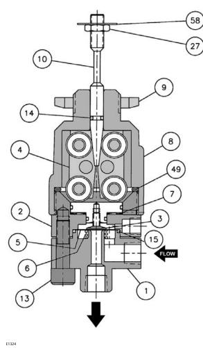
Figure 6. Baumann 81000 NPS 1/4 Angle Valve Body
