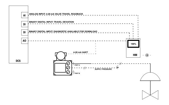
Figure 3. Using the HIM in a Conventional Analog Control System
