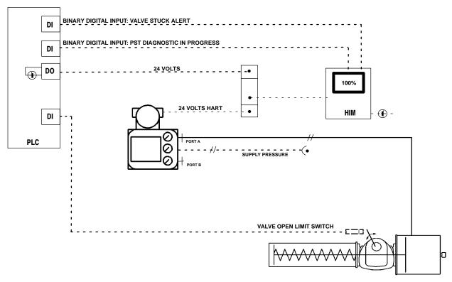
Figure 4. Using the HIM in a Safety Control System
