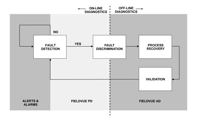
Figure 2. Four Phases of Valve Diagnostics
