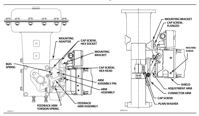
Pneumatic tubing connected to the DVC6000 brings instrument supply air to the DVC6000 and takes controlled output air from the DVC6000 to the actuator. Pressure sensors in the DVC6000 measure these pressure signals and present them as device variables.
