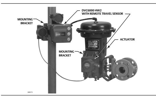
Pneumatic tubing connected to the DVC6000 HW2 brings instrument supply air to the DVC6000 HW2 and takes controlled output air from the DVC6000 HW2 to the actuator. Pressure sensors in the DVC6000 HW2 measure these pressure signals and present them as device variables
