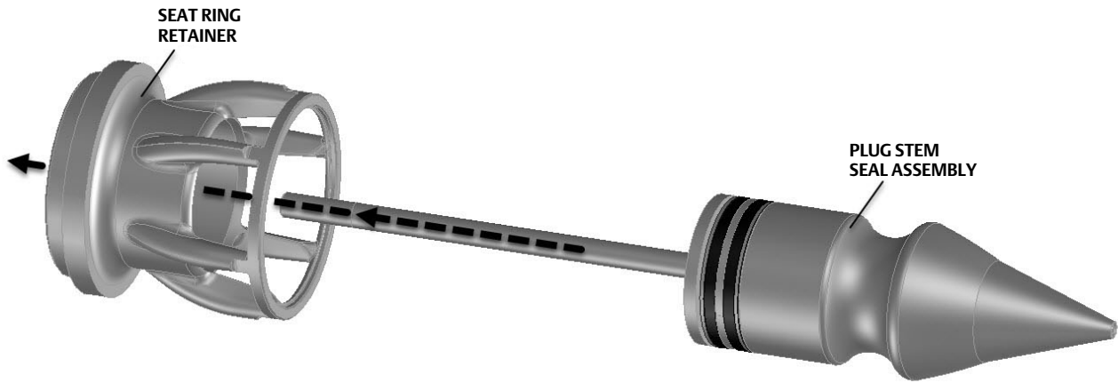
Figure 11. CCV-N NPS 4 Assembly for Application Up to and Including 316°C (600°F) (Except Bore-Seal Trim) — Insert of Plug Stem Seal Assembly through the Bottom of the Seat Ring Retainer
