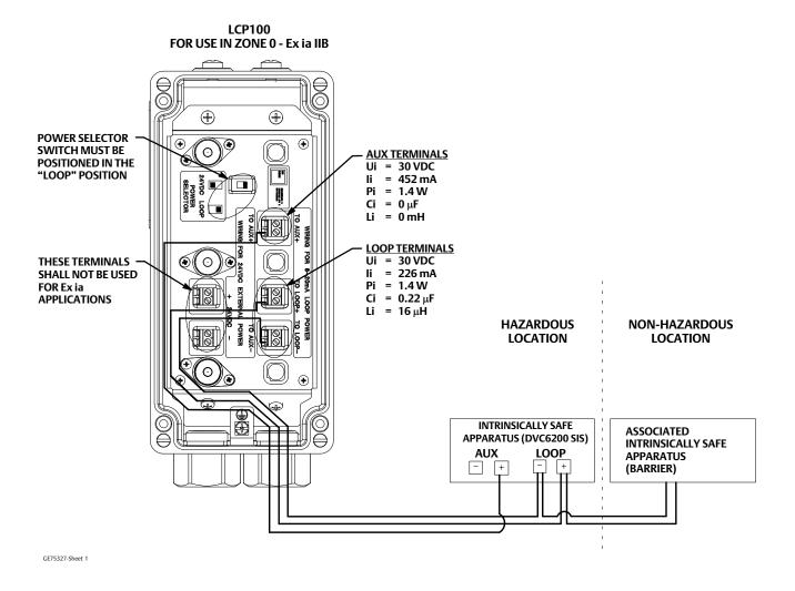
Figure 3. Schematic Notes for Figure 2 and Figure 4
