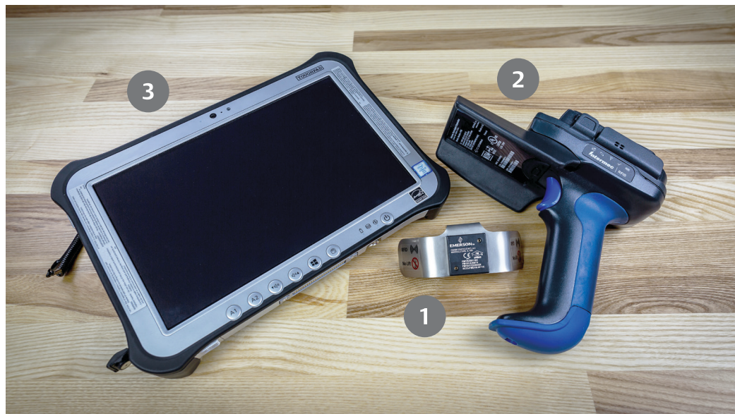
Figure 1 Equipment for reading/writing an Asset Management Tag
