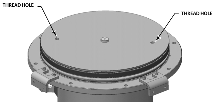
Figure 21. Threaded Holes in Pneumatic Cylinder
