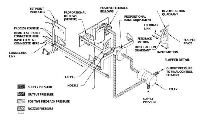
As the process temperature decreases, approaching the lower switching point, the flapper moves away from the nozzle (in a direct-acting controller), reducing nozzle pressure. Through relay action, pressure to the positive feedback bellows is reduced, moving the flapper further away from the nozzle. Thus, the nozzle pressure falls even further. Output pressure to the final control element switches to zero.
