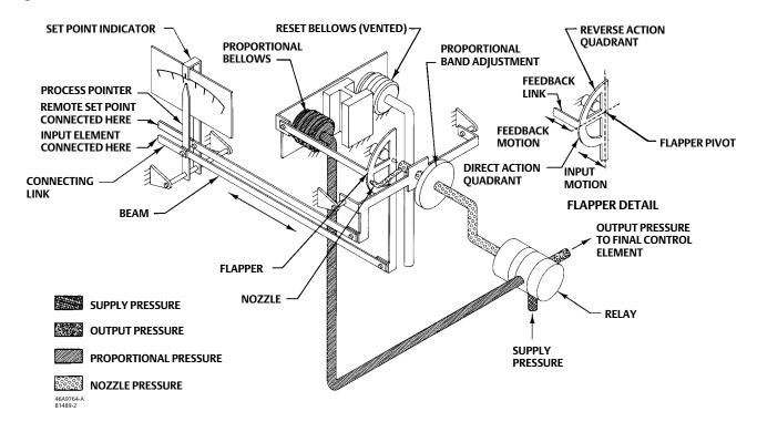
Moving the set point indicator changes the distance between the nozzle and flapper as does a change in process temperature except that, when the set point is changed, the nozzle moves with respect to the flapper.
