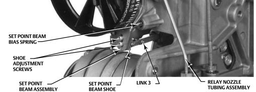
ASSEMBLED VIEW (CONTROLLER REMOVED FROM CASE)
