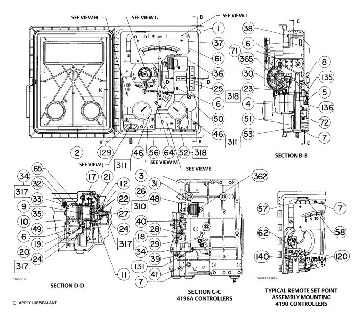
Figure 48. Controller Assembly Drawing (cont'd)
