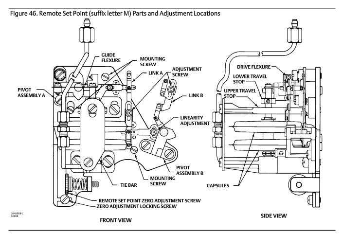
Replacing Pivot Assembly A (Key 114)
