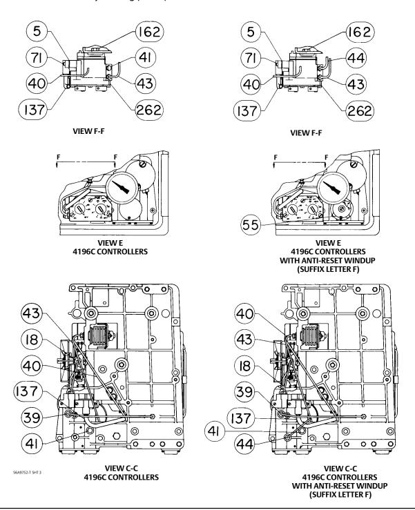
Figure 48. Controller Assembly Drawing (cont'd)
