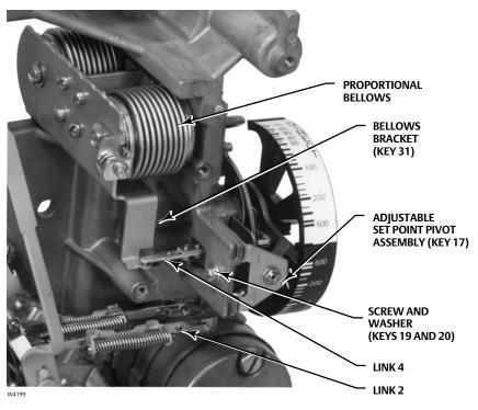
11. Disconnect link 4 from the bellows bracket (key 31). Refer to figure 35 for the link location.
