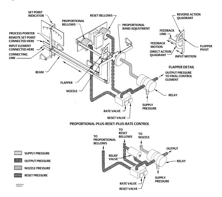
PROPORTIONAL-PLUS-RESET-PLUS-RATE CONTROL WITH ANTI-RESET WINDUP
