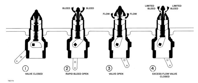
Figure 2. Operational Schematic
