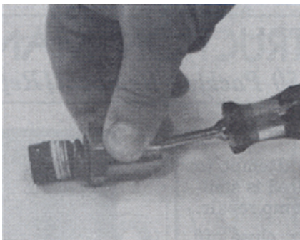
Figure 6. Remove packing carefully (step 8)
