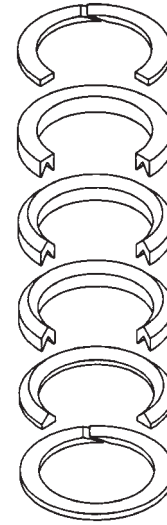
STACKING ORDER OF PTFE PACKING RINGS
