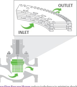
Unique Flow Passage Shapes reduce turbulence to minimize shockassociated noise and place turbulent shear layers away from solid boundaries to reduce noise. The multi-stage pressure reduction, utilized with sound engineering principles, controls jet size, formation, interaction, and accommodates fluid expansion.
