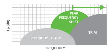
Frequency Spectrum Shifting reduces strain and acoustic energy in piping by exploiting the natural damping of high frequency acoustic waves. Piping transmission loss is maximized to reduce radiated aerodynamic noise.
