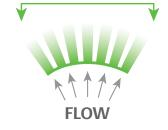
**Exit Jet Independence** is crucial for avoiding jet coalescence, which will lead to additional noise. All Emerson noise technologies are designed with this critical factor as standard.
