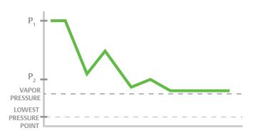
Cavitation Prevention is possible as the liquid undergoes a portion of the total pressure drop in each stage. This prevents the liquid in any stage from falling to or below its vapor pressure, avoiding cavitation.
