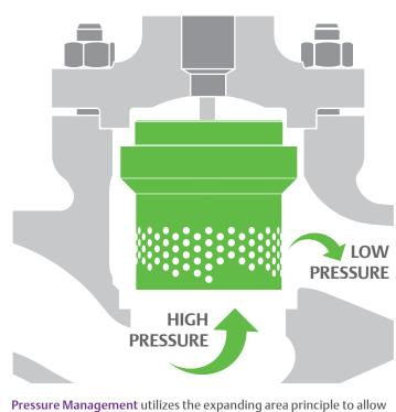
Pressure Management utilizes the expanding area principle to allow for volumetric expansion of depressurizing gas and safe pressure reduction of potentially cavitation liquids.
