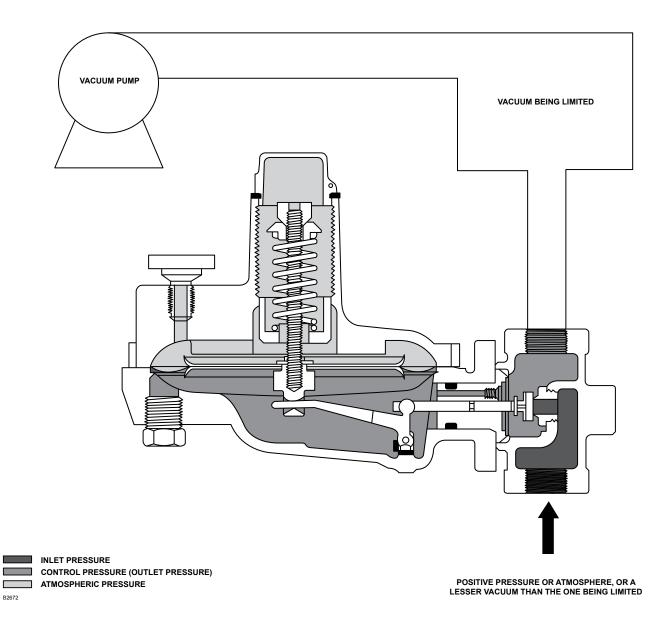
Figure 2. Y690VB Series Operational Schematic
