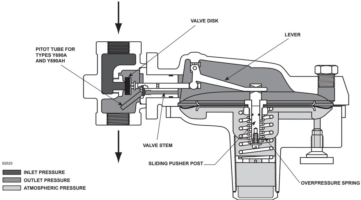
Figure 2. Y690A Series Operational Schematic
