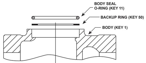
**Figure 4.** Expanded View of the Body Area Showing the O-ring and Backup Ring Placement
