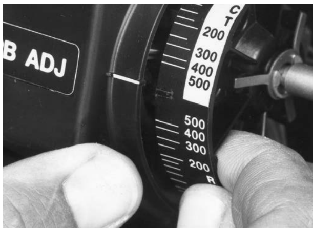
Figure 3-2. Changing Controller Action on Fisher 4195KA Controllers
