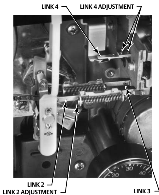
Figure 6-10. Link 2 and 4 Adjustment Locations
