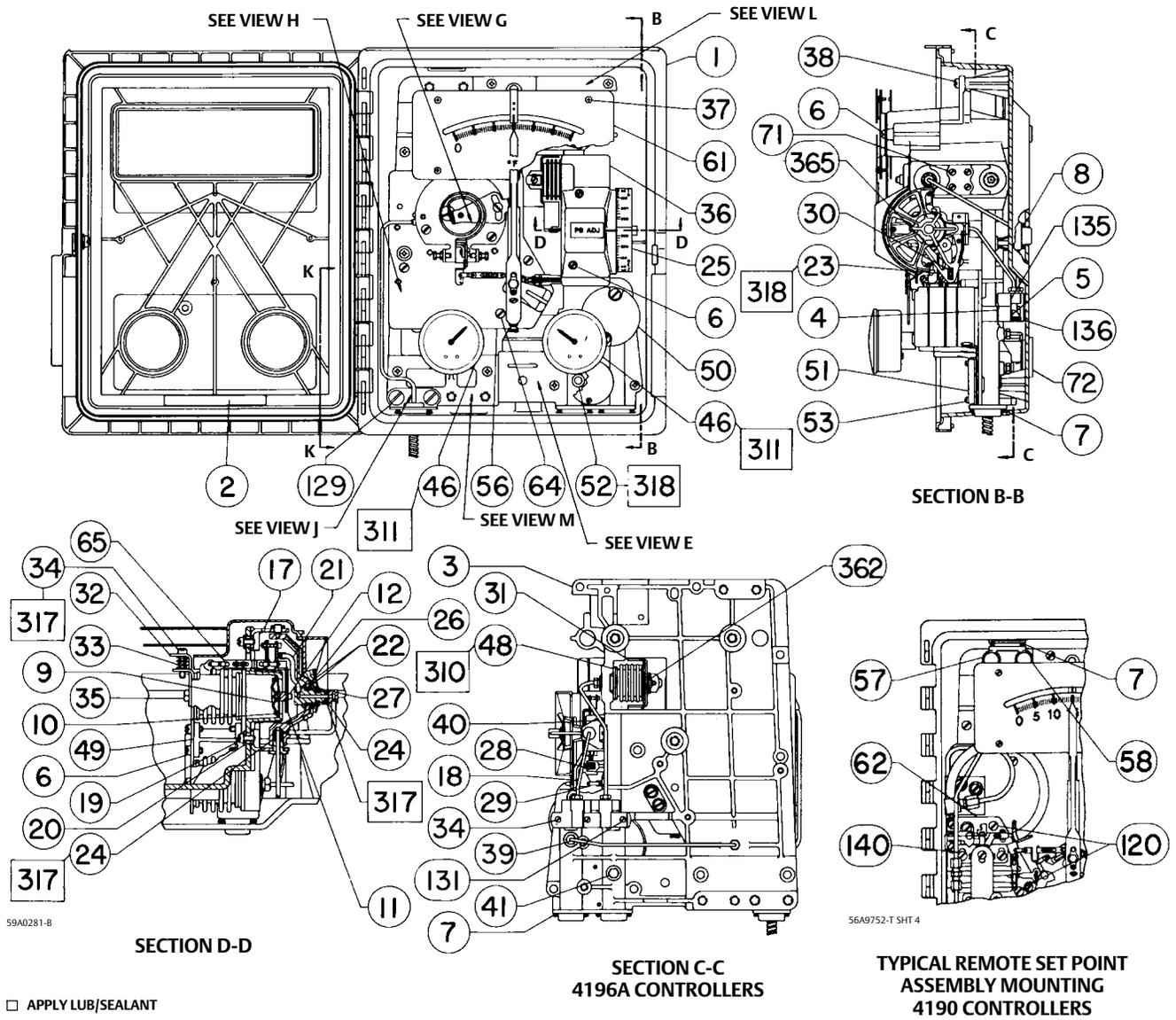
Figure 48. Controller Assembly Drawing (cont'd)
