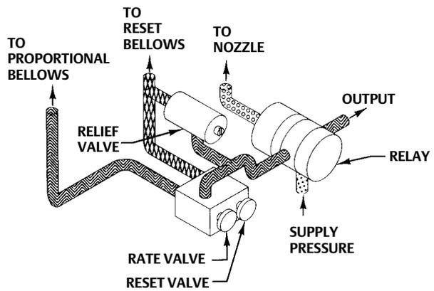
PROPORTIONAL-PLUS-RESET-PLUS-RATE CONTROL WITH ANTI-RESET WINDUP
