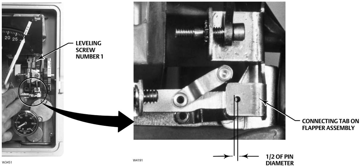
24. Set the proportional band between DIRECT and REVERSE. Do this by aligning the tab on the proportional band adjustment knob with the hole in the set point beam assembly as shown in figure 32.
