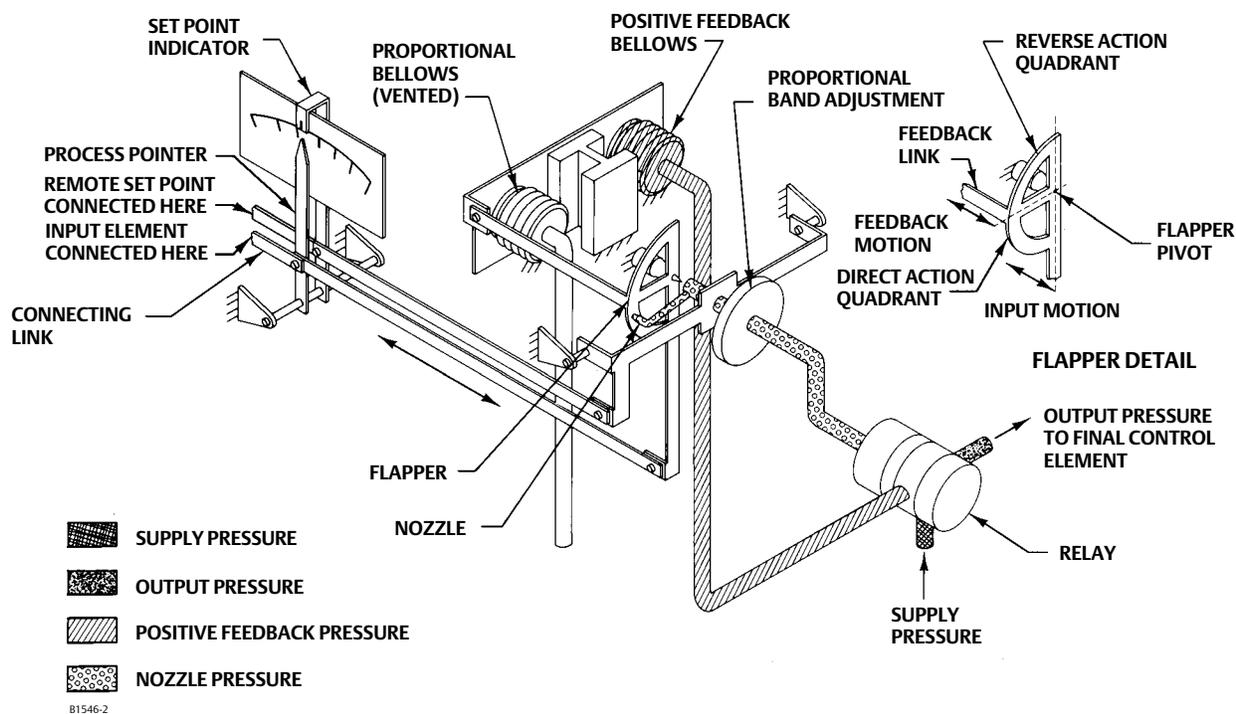
As the process temperature decreases, approaching the lower switching point, the flapper moves away from the nozzle (in a direct-acting controller), reducing nozzle pressure. Through relay action, pressure to the positive feedback bellows is reduced, moving the flapper further away from the nozzle. Thus, the nozzle pressure falls even further. Output pressure to the final control element switches to zero.
