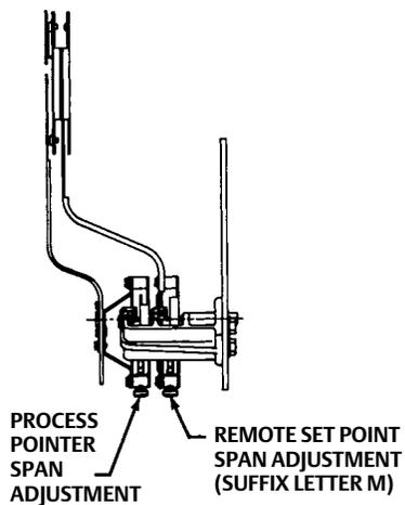
SIDE VIEW OF SET POINT/PROCESS INDICATOR ASSEMBLY
