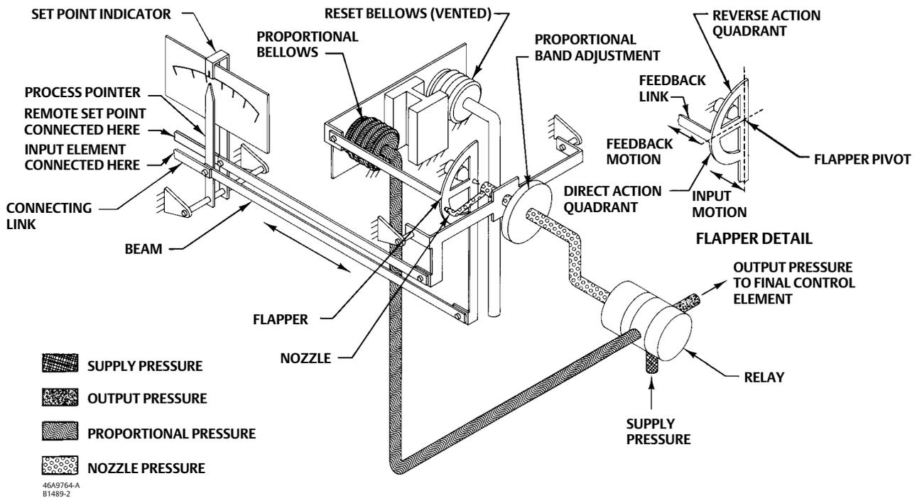
Moving the set point indicator changes the distance between the nozzle and flapper as does a change in process temperature except that, when the set point is changed, the nozzle moves with respect to the flapper.
