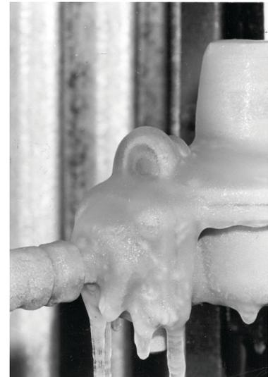
VENTS ON HORIZONTALLY MOUNTED REGULATORS BECAME QUICKLY PLUGGED DURING FISHER'S TESTS.
