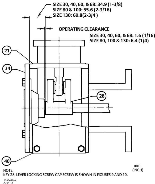
12. To aid installation of the lever, apply lithium grease lubricant (key 93) to the valve shaft spline.
