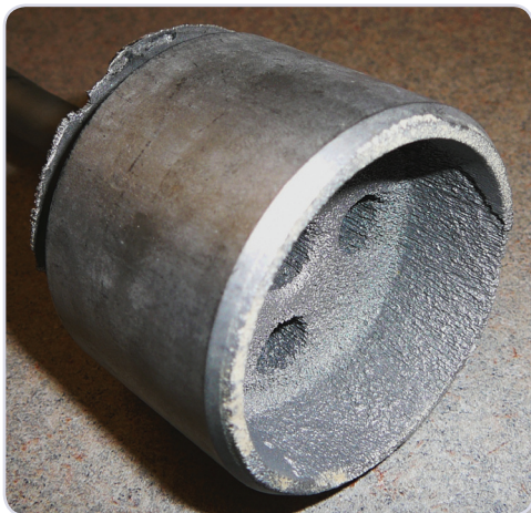
Type 316 stainless steel plug showing severe corrosion
